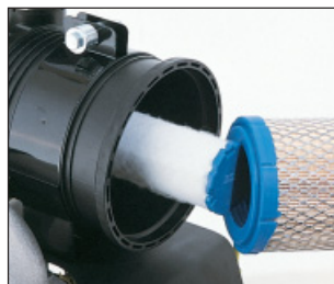
Air cleaner has two filters: the main filter traps dirt while the inner filter prevents carburetor contamination during main filter servicing.
