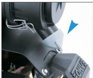
Ejector valve on air cleaner continuously eliminates dust that swirls inside the air cleaner canister.
